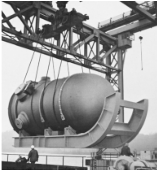
◀ The United States no longer has the capability to build nuclear pressure vessels. This stainless steel pressure vessel was designed and fabricated by Combustion Engineering in the late 1970s.
