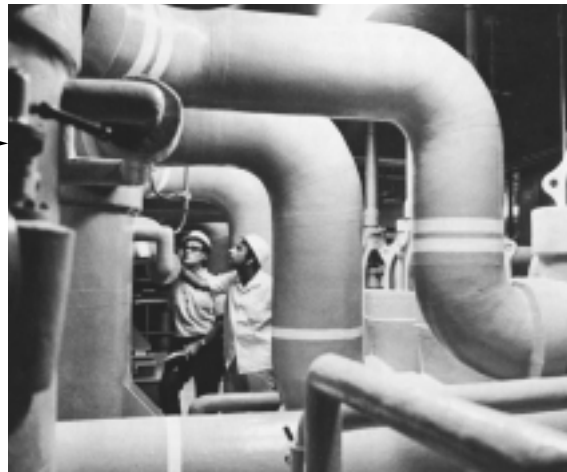
▲ A high-capacity coolant pump, produced by C-E/KSB Pump Company in the late 1970s. The pump was assembled and tested in a full-flow loop at the manufacturing facility, before being shipped to the nuclear reactor site.
